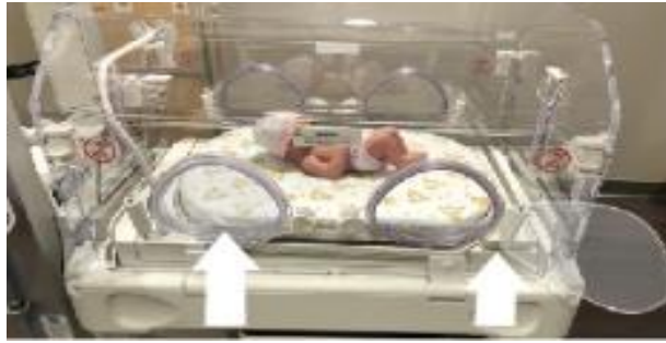
Figure 3. LATCHED (left) and UNLATCHED (right) portholes
