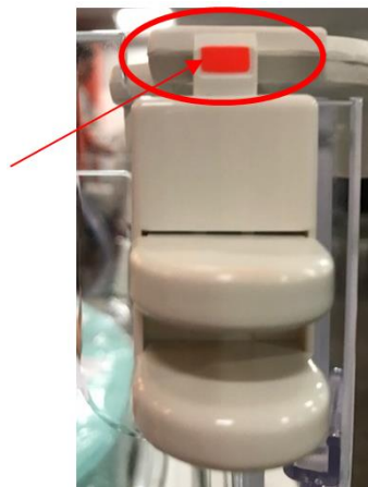
Figure 1. UNLATCHED bedside panel The red tab shows the latch is not engaged.
