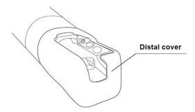
8 Confirm that there is no adhesion of foreign materials between the distal end of the endoscope and the distal cover.
