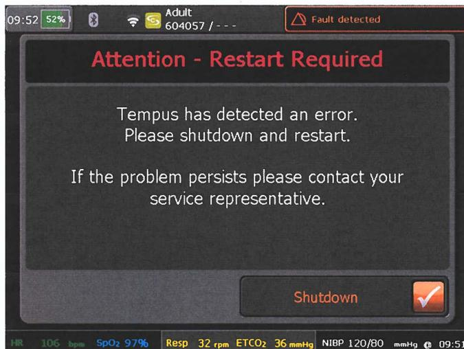
If this error occurs, the pulse tone (audio) that reflects the patient's level of oxygen saturation is no longer sounded. Additionally, the user will no longer be able to visualize the airway requiring the user to either intubate the patient without video imaging or use an alternative laryngoscope not connected to the Tempus Pro Monitor. This message cannot be cleared from the Tempus Pro Monitor's screen, and
