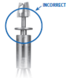
Fig. 5 Backup Milling Assembly (INCORRECT)
