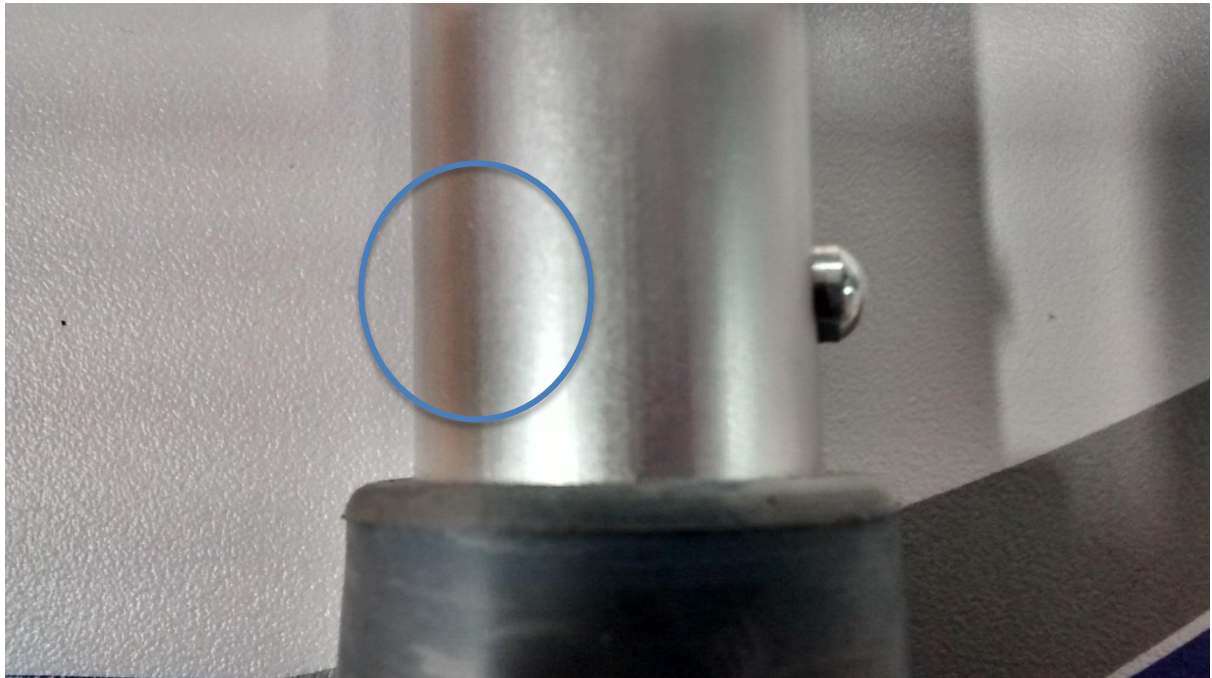
Image 2 – One spring clip pin missing
