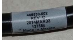
Figure 1 Improperly assembled power cord, falls in date range
