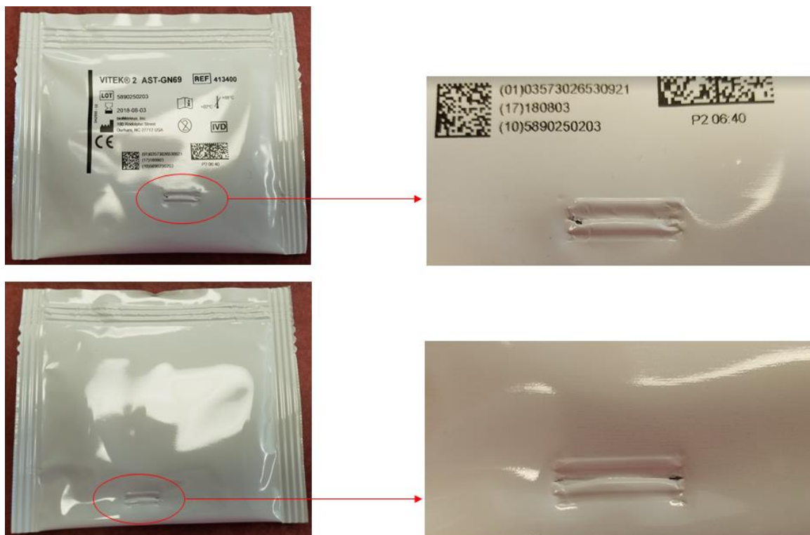
Figure A - Example of Pouch Defect
