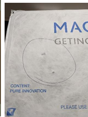
Picture 3: example of holes in the Tyvek cover
