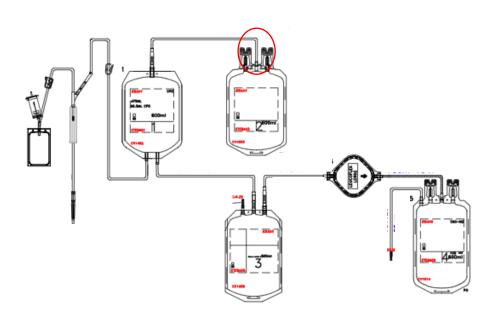
Traceability of the defective bags (CV1003) highlights a unique day of production (21/12/22) during a specific period of the day and coming from a unique welding machine (A3).
