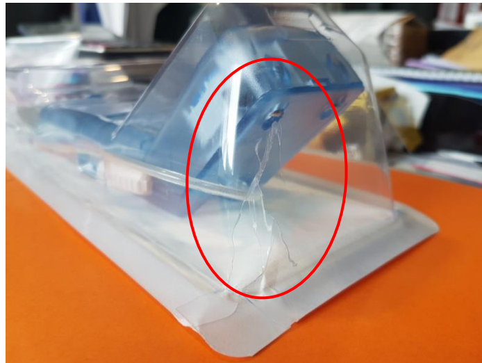
Picture 2: Example of crack observed near the inflation device pressure gauge
