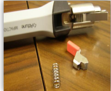
Figure 3: Fractured ATTUNE® INTUITION™ Impaction Handle
