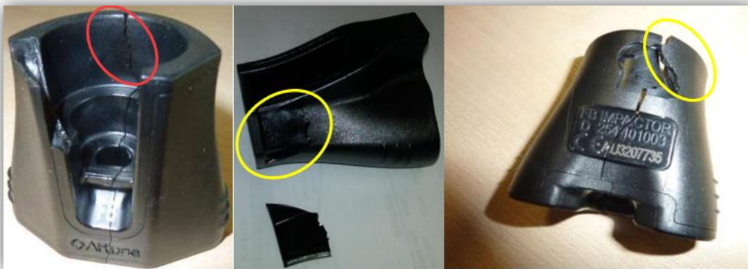
Figure 4: Fractured ATTUNE® INTUITION™ Impactors
