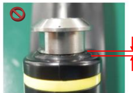
Picture 03: The rubber part lifted
