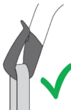
PICTURE 2 - CORRECT SLING LOOP ATTACHMENT
