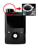
The images show a **normal** pump retainer ring vs a **damaged or missing** pump retainer ring.
