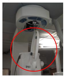
Figure 1: Example of a detached L-arm rotation cover
