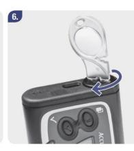
Use the battery key to fully tighten the battery cover. You can verify that the battery cover is correctly tightened by checking that it is in line with the pump casing. Do not over-tighten.
