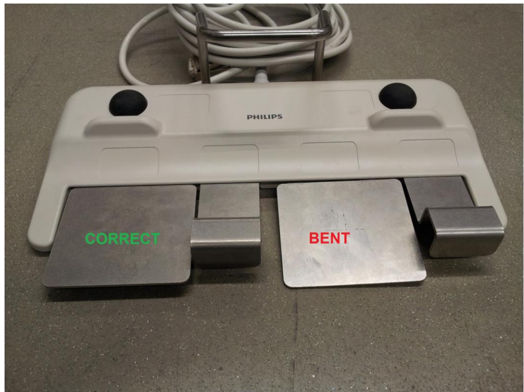
Left pedal is correct. Third pedal from left is bent. Distance to floor should be approx. 12mm or 0,47inch.
