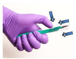
**Step 2: Expose the Blade -** Depress the top button on the clear protective shield and **retract** the protective shield to the rear locked position to fully uncover the blade.
