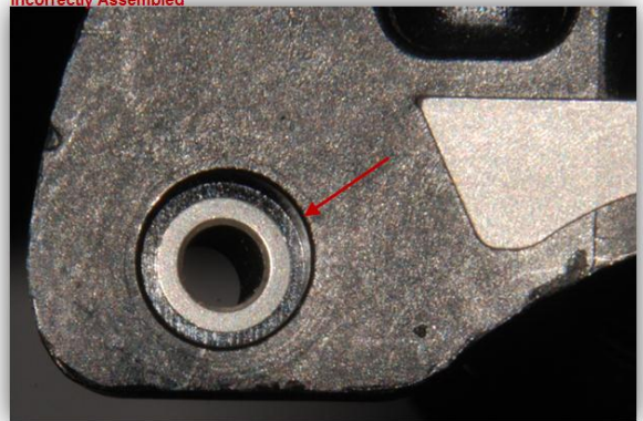
Figure 3: Bottom of Jig (bone side) – Comparison of Correctly Assembled vs. Incorrectly Assembled (Inverted Bushing)
