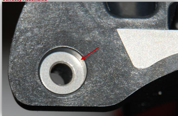
Figure 3: Bottom of Jig (bone side) – Comparison of Correctly Assembled vs. Incorrectly Assembled (Inverted Bushing)
