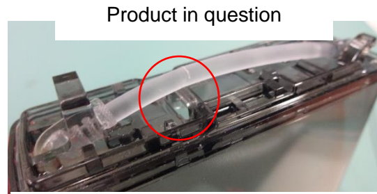
Arch on the pressure plate and pumping tube is pushed up over the arch
