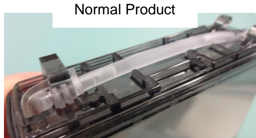
Pressure Plate has tunnel for pumping tube
