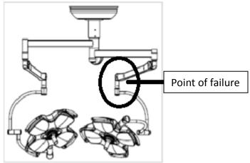
This potential for malfunction is caused by fissures near the weld seam at the front pivot of the spring arm. The design of the spring arm was improved in 2006. The devices involved for your market are limited to those listed in the attached Consignee list.
