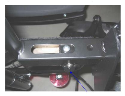
2.1 Below is a more detailed picture on the screw that you have to loosen with an Allen key.
