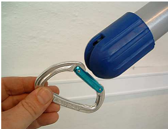
3) Hold the carabiner like shown, with its opening pointed towards the cross pin of the lifting arm. (Widest part of carabiner pointing upwards).
