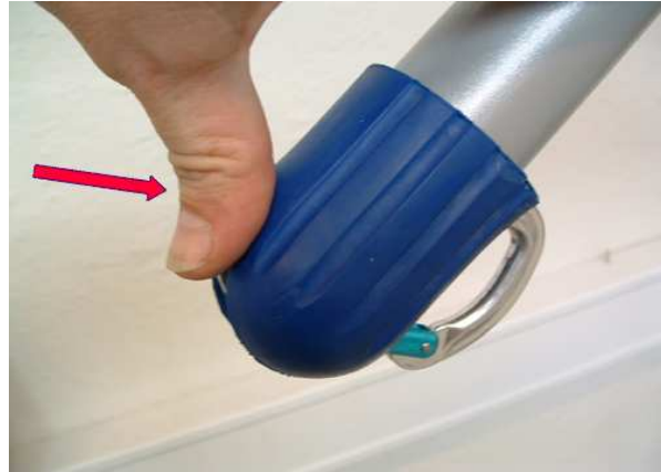
6) Turning the carabiner all the way around the cross pin. (Because of friction between the rubber protection and the carabiner, considerable force may be applied when performing this step.)
