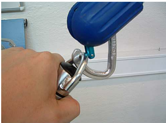
9) Attaching the spreader bar to the carabiner.
