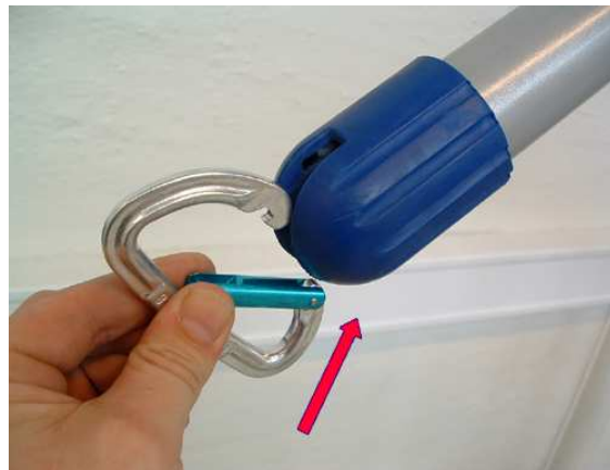
4) Open the safety catch by use of two fingers and press upper part of the carabiner around the cross pin.
