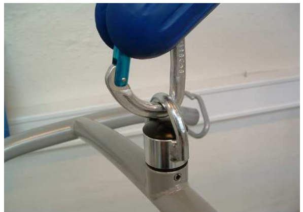
10) Correctly attached spreader bar .
