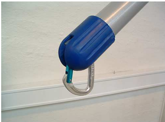
7) Carabiner correctly positioned on the lifting arm, ready for use.
