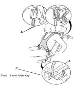
This item should be fitted by an experienced clinican or technician. The harness must always be used in combination with the pelvic belt and should be worn on top of the pelvic belt. Make sure that the harness does not put too much pressure on any point.
