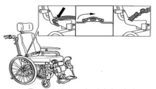
The pelvic belt is mounted on the backrest brackets. Thread the belt through the mounting on the chair and then through the two plastic buckles as shown in the picture. It is important that both buckles are used. There is a danger the belt might slip if the belt is threaded through only one.
