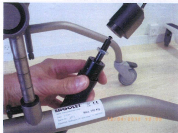
6. Remove the old gas spring.
