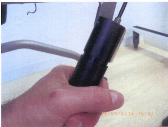
13. Press the cover tube on to the Plastic housing.
