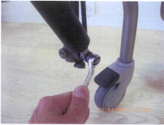
3. Unscrew the M8 lock nut.
