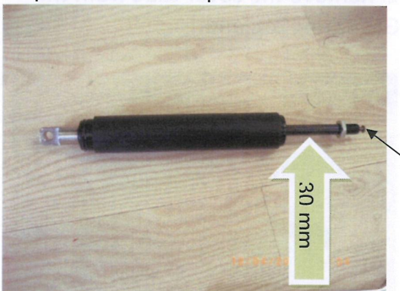
7. Fit the cover tube to the new gas spring in the same direction as on the old gas spring. Release the gas spring to have 30mm free piston rod.
