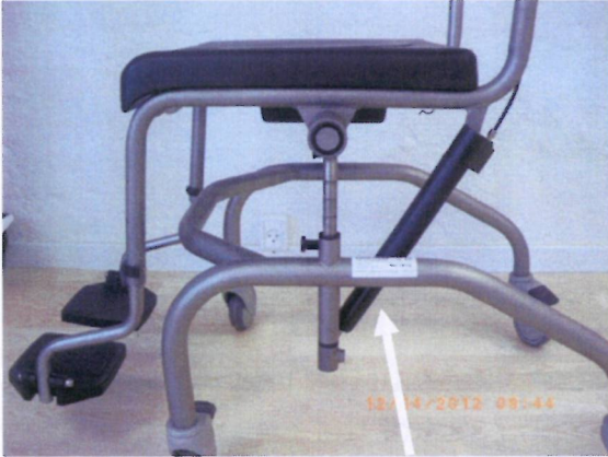
Gas spring to be replaced.
