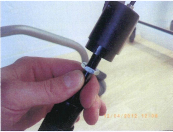
9. Cut the plastic strip and fit the piston rod end to the housing.
