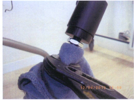
10. Screw in the piston rod until the gas spring is released. Use the cloth to protect the piston rod from scratches.
