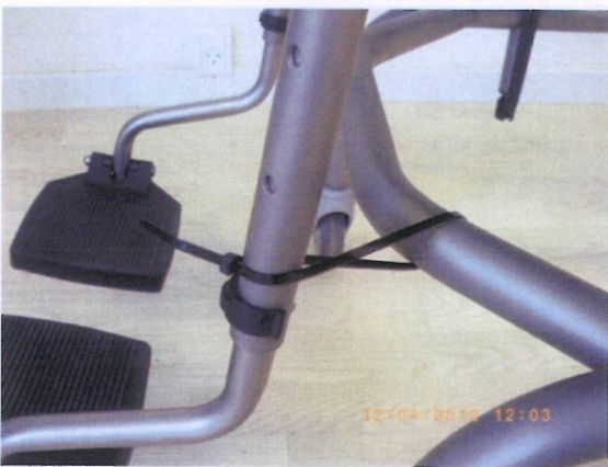
5. Lock the tilt function with a plastic strip to make the replacement easier.
