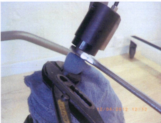
11. Unscrew the piston rod 1 turn* and tighten the M10 nut whilst securing the piston rod.
