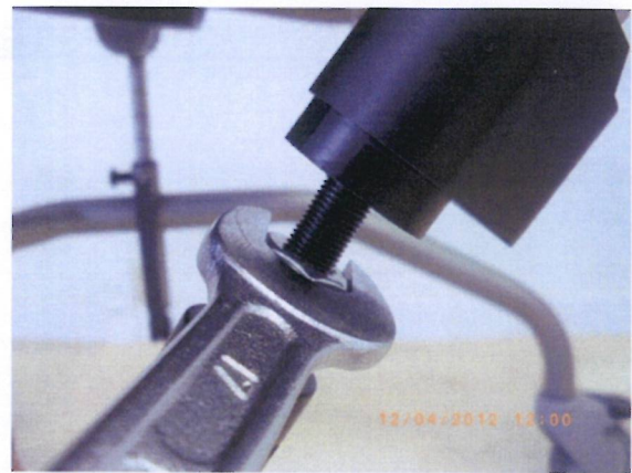
4. Unscrew the M10 nut. Keep unscrewing until the piston rod thread has come out of the plastic housing.
