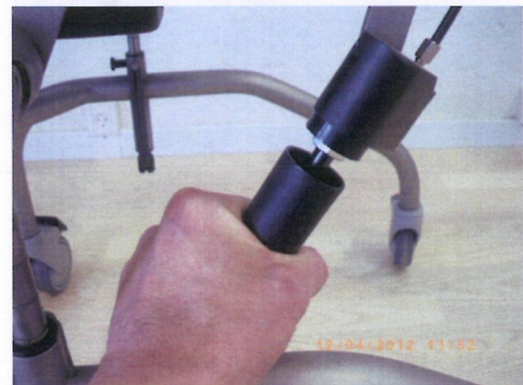
1. Remove the cover tube from the Gas spring top end.
