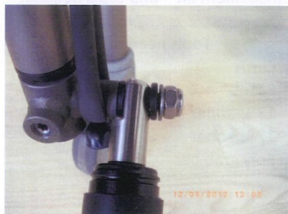
8. Fit the gas spring to the threaded tap at the bottom end.
