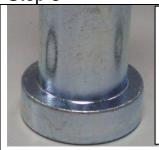
Check the shoulder of the pivot pin for wear. Nominal thickness is 10mm.
