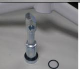
Remove the O-ring and extract the pivot pin from the spreader bar
