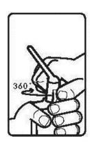
2. To break the seal twist the nozzle clockwise one full turn (the nozzle should then be in the same direction as before turning).
