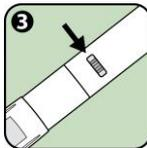
3. Make sure that the **injection indicator** is not red. If it is red, this means that the Anapen Auto-Injector has already been fired and you must discard it.
