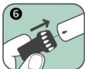
6. After the injection, the needle sticks out. To cover it, click the wide end of the black needle shield back on the open end (needle end) of Anapen Auto-Injector (as indicated by the arrow).
