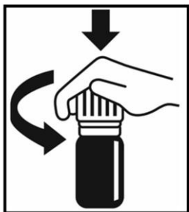
1. Opening of the child-resistant closure: Push down and turn.
