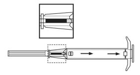
3. Pull the plunger of the applicator completely backwards until you can see a complete line in the second window.
