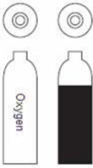
The colour coding of the shoulders of Compressed Medical Oxygen cylinders is white (RAL 9010).
