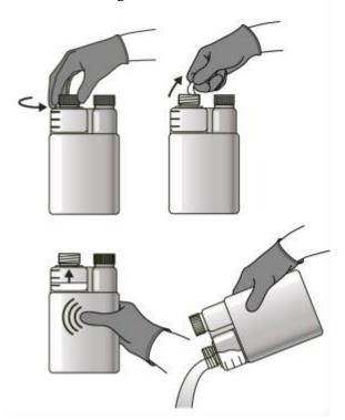
2. Attaching the 1 and 2.5 litre containers to the appropriate applicator:
