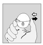
1. To release the dust cap press the piercing button completely in and let go.
