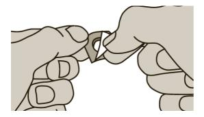
2. The foil is easily peelable. Do not force the wafer through the foil as it is fragile and can easily break. Instead, fold back the foil and then peel it off.
