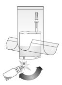
Break open the mechanism in the tube of the vial connector by repeated bending backwards and forwards. This establishes the connection. Please hold the tube – and not the vial – during this process!
