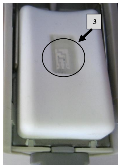
Figure 6 Counterfeit product with no visible cables
