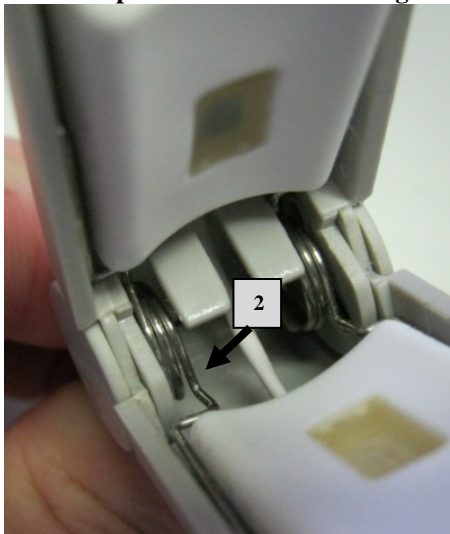
Figure 4 Counterfeit product with 3 windings of the feather
