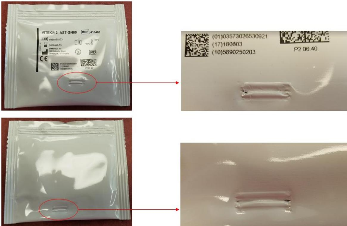
The root cause of this issue has been identified and corrective measures have been taken to ensure issues of this type do not affect future Manufacturing lots. Card lots manufactured after March 16, 2017 include a new stitch seal (see Figure B below) and are not affected by the described issue.
