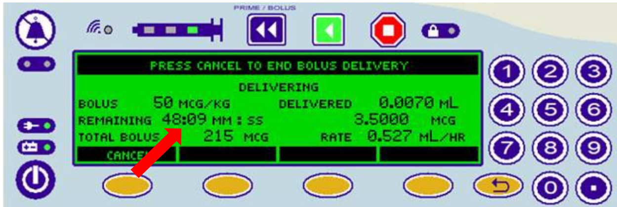
Figure 4: Example of Incorrect Time Remaining. “REMAINING 48:09 MM:SS” should be displayed as “REMAINING 04:09 MM:SS”
