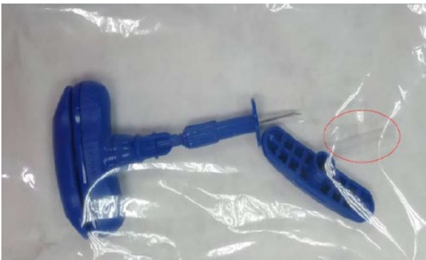
Figure 1: Needle Protector Dislodgement
