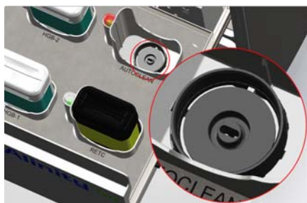
Drawings of Alinity hq Autoclean Solution bottle holder showing detail when the safety interlock covers the piercing probes and when the safety interlock does not deploy showing the exposed piercing probes. All bottle holders have identical piercing probes.
