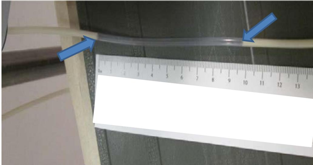
\*This is an example and the air in the tubing may not be as pronounced as shown in the image.
