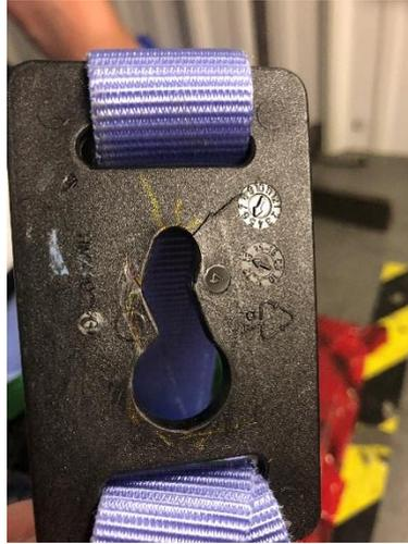
Image 2: Picture of a broken sling clip
