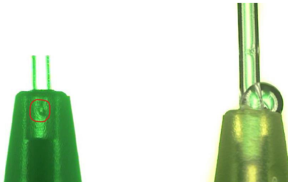
Figure 1. 24GA Jelco showing catheter hole circled in red causing leakage
