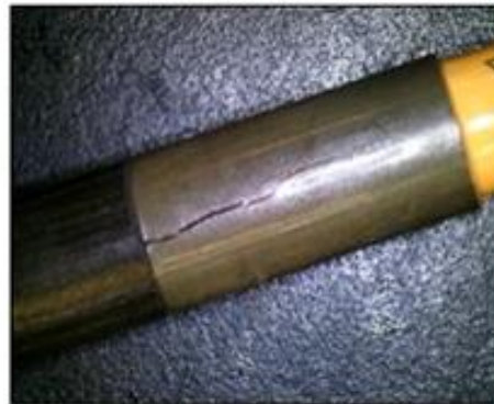
Figure 2. Example of crack found on damaged MCS instruments
