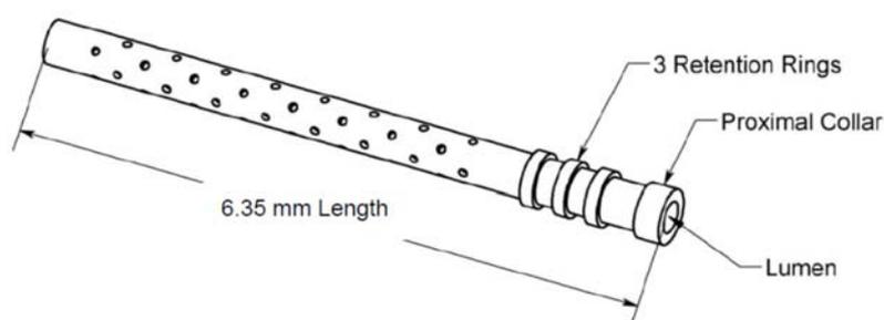
**Figure 1: CyPass Micro-Stent**
