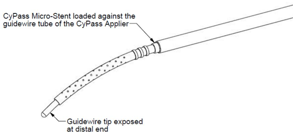
**Figure 4: CyPass® Micro-Stent loaded onto CyPass® applier guidewire**
