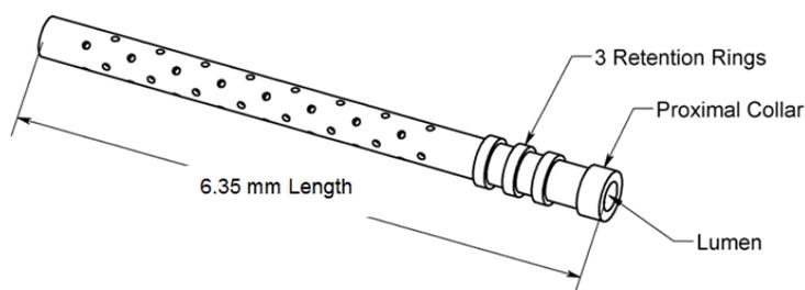
**Figure 1: CyPass® Micro-Stent**
