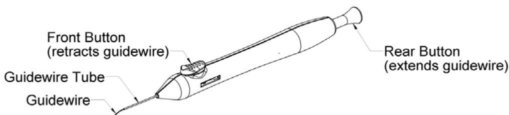
**Figure 2: CyPass® applicator with Guidewire Extended**
