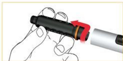
Insert the new cartridge into the cartridge sleeve.
